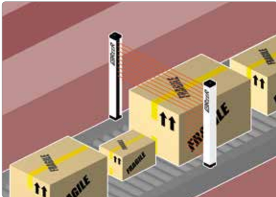
Measurement of the height of objects in transit on conveyor systems
